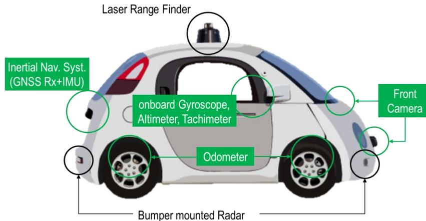
**Figure 1. Sensors embedded in cars useful for positioning, in green those considered as the most easily accessible. The Google car is only used for illustration purposes.**
