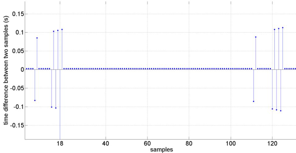
**Figure 6. Time interval between two consecutive time stamps of the hybrid receiver MTi position estimates.**
