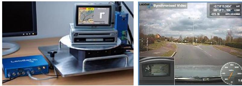
Figure 2. LabSat Turntable System and visual assessment of the position performances based on recorded vehicle's data [5]
