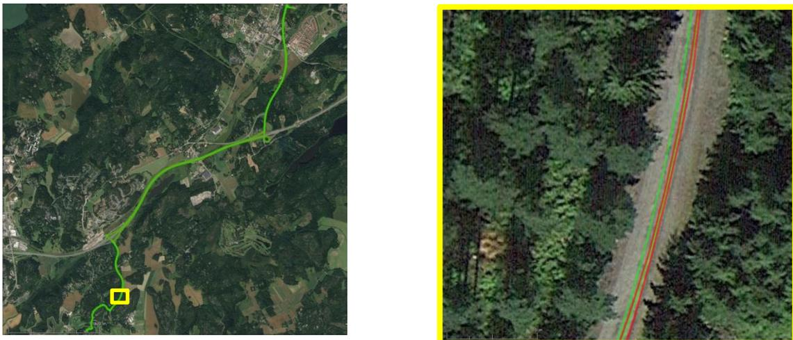
Figure 5. Reference (green) and hybrid receiver (red) trajectories with a zoom (yellow) in the forest.
